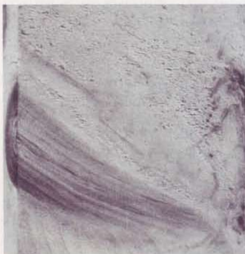
Sound, tight (intergrown), spiked red knot.
